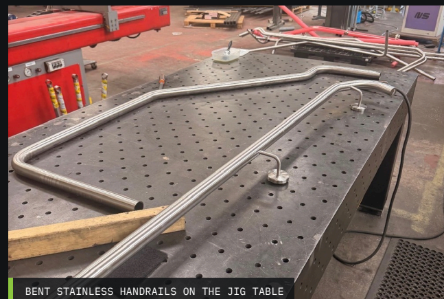
BENT STAINLESS HANDRAILS ON THE JIG TABLE
